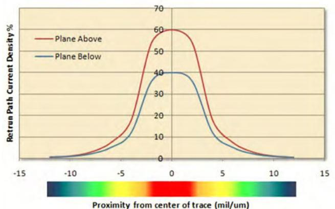
Figure 3: Return path current density for asymmetric stripline (source: iCD Design Integrity).
