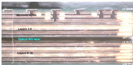
Figure 4: PhoxDem09.04MPX – 18L+2 opt embedded WG layers.
