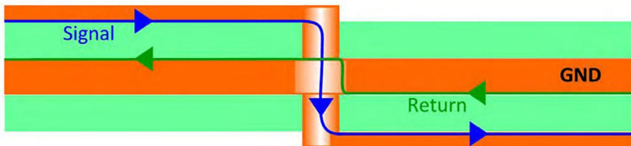
Figure 4: Central GND plane return path structure.
