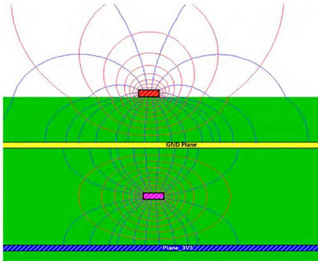
Figure 2: Electric (blue) and magnetic (red) fields (source: HyperLynx).
