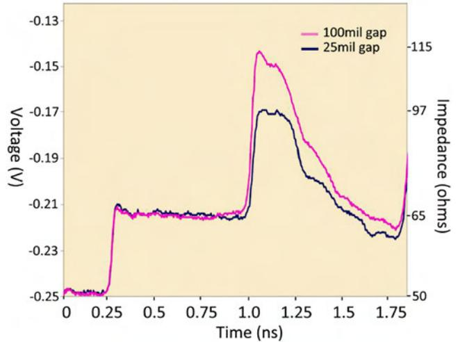
Figure 1: Inductive spike for 25 & 100 mil gaps (source: Byers).
