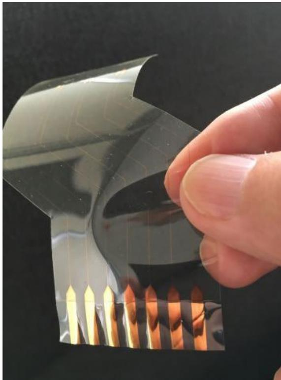
Figure 1: Transparent/flexible circuit example.
