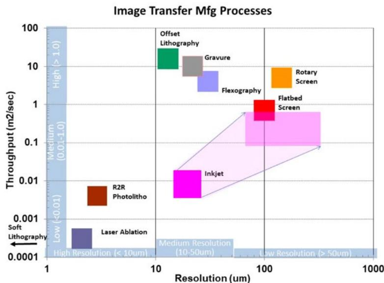
Figure 2: Printing techniques compared by resolution versus throughput. Arrow indicates soft lithography as a photoimageable technique that is off the scale to the left<sup>3</sup>.
