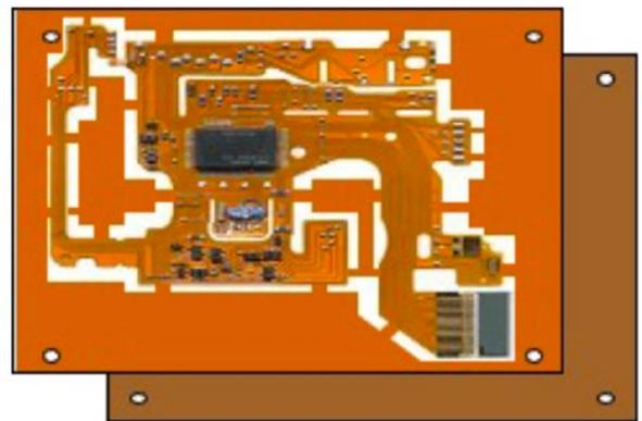
Figure 2: Flexible circuit retained in a uniform panel format.
