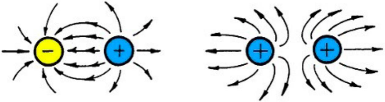
Figure 1: Electric lines of force (field) illustrate Coulomb's Law.
