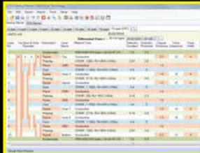
Stackup Impedance Analysis, Single-ended, Differential Pairs and CPW Blind and Buried Via Definition, Reference Plane Assignment Validation
