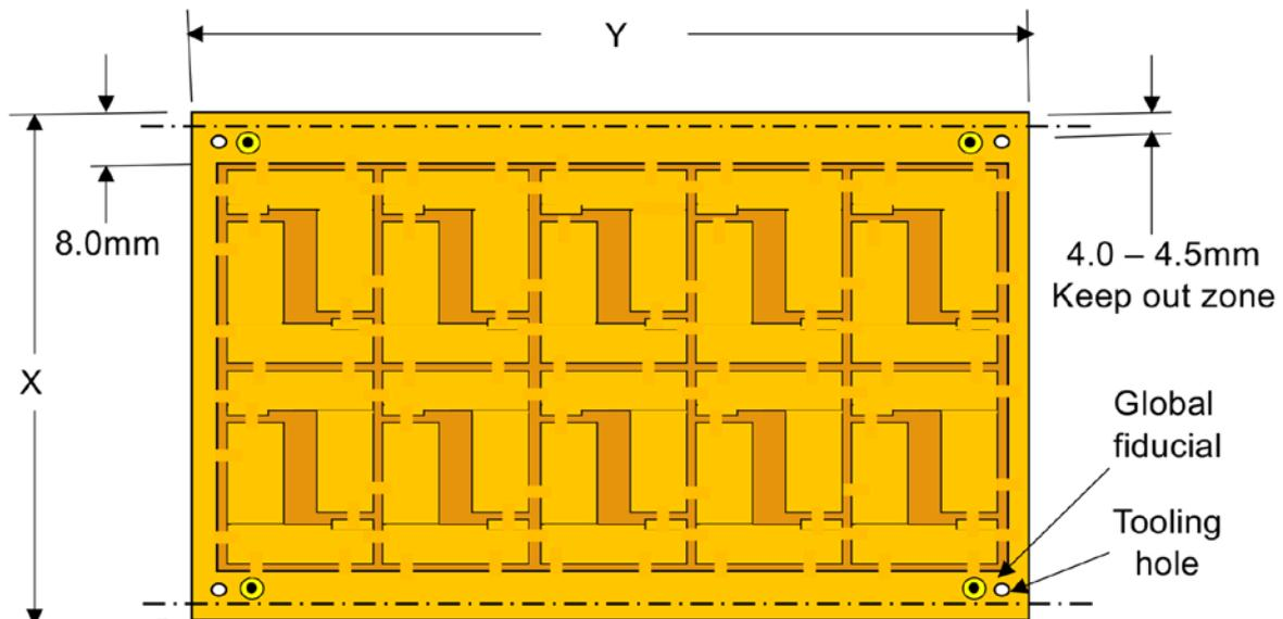
Figure 3. Opposing orientation array format.
