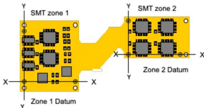
Figure 4. Fiducial target location for two component mounting zones.
