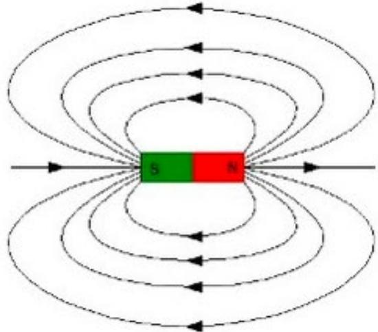
Figure 3: Magnetic lines of force (field).
