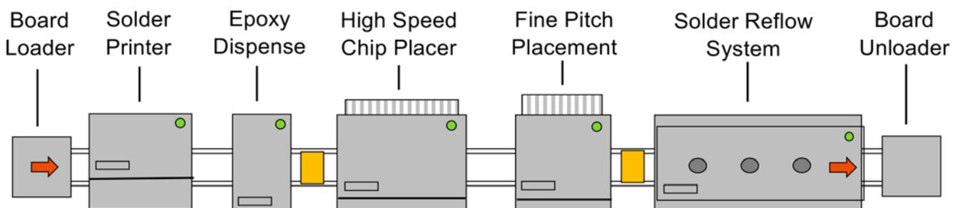
Figure 1: Basic conveyorized SMT assembly line configuration.
